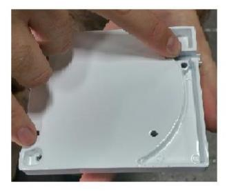
Locate small spline in the channel
