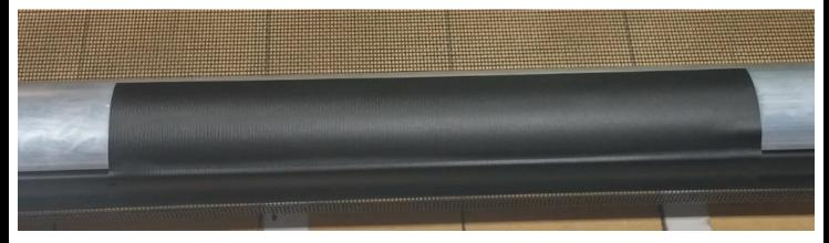
Place the spring in the upper endcap, re-attach the endcaps, and feed the mesh into the endcaps
