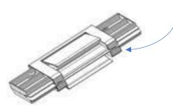
Unscrew the 2 small 2mm Allen screws (one on each side, one at the bottom and one at the top)
