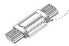
Unscrew the 2 small 2mm Allen screws (one on each side, one at the bottom and one at the top)
