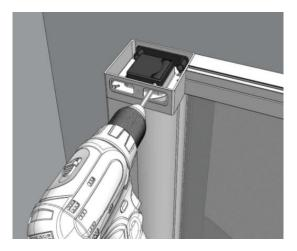
Do not rotate at full speed of drill as this will cause gears to overheat. Use low gear on drill. Caution: Do not over tension! Never apply more than 100 turns to the Spring. 20:1 gear ratio (20 turns on gearbox = 1 on spring)
