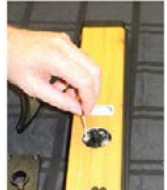
Remove the lower endcap, the back of the handle and remove brake rod assembly from the bottom
