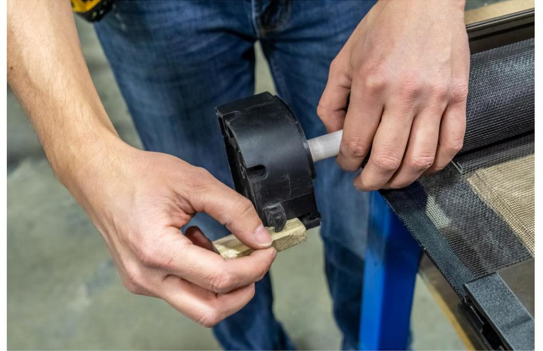
Place the endcap on the spring end and wind as per the turn guide on next page for direction and number of turns
