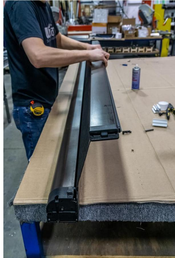
Once cap is on, bench test screen for tension
