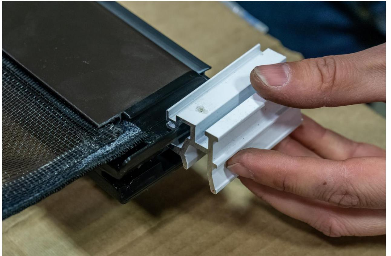
Position small piece of track on end of pull bar
