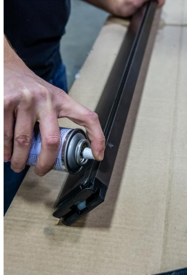
Carefully feed the spline back onto the pull-bar
