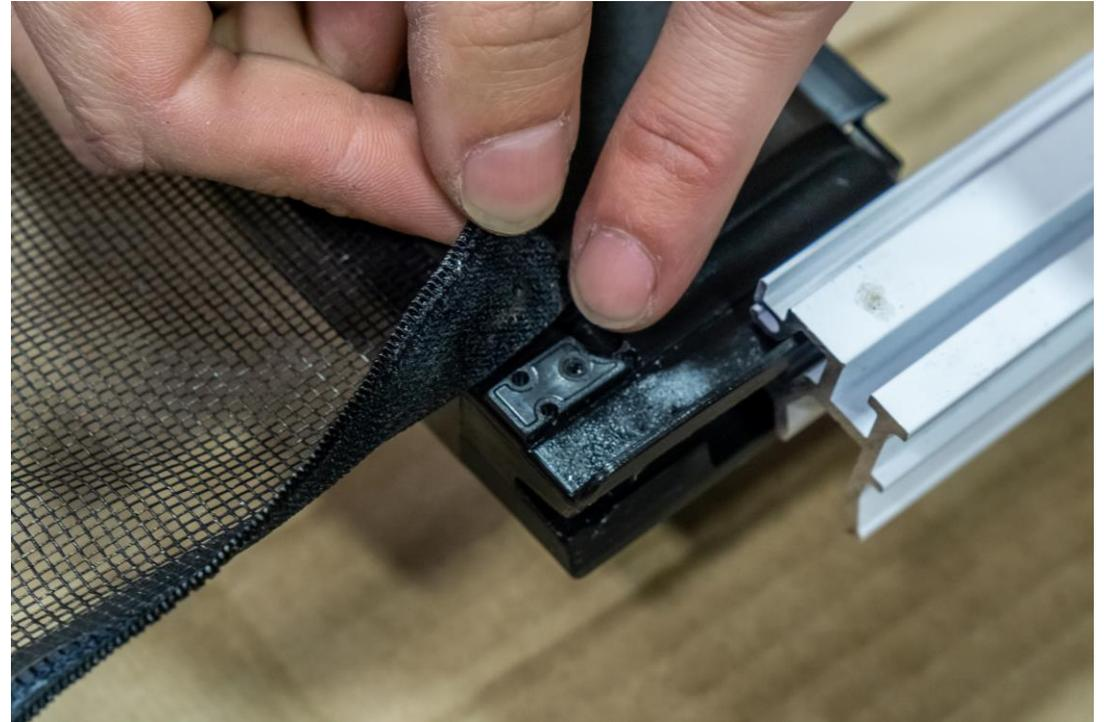
Feed mesh into track piece to ensure the mesh is positioned correctly before installing the two mesh retainers
