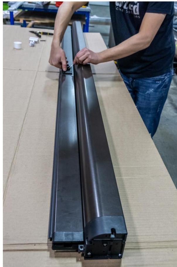
Put the rivet in a handle to release the brakes for RE-installation
