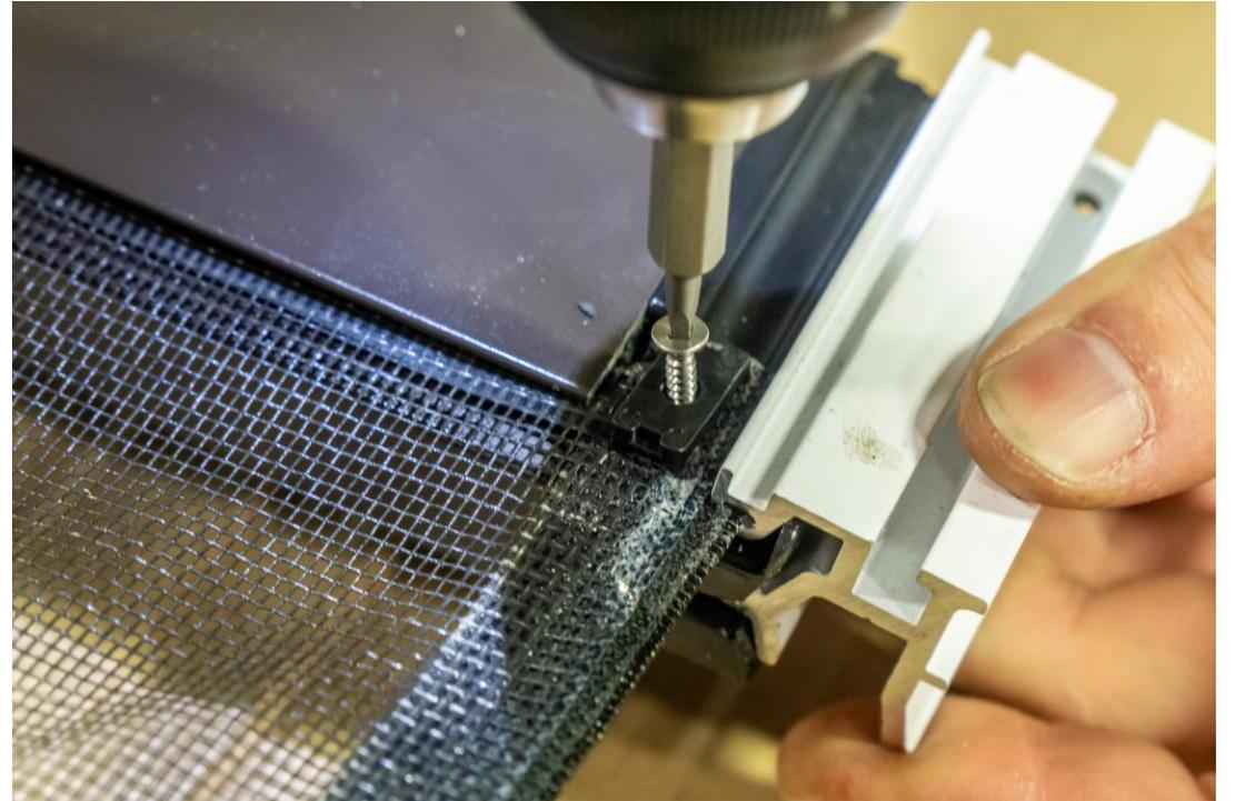
Roll the mesh up and insert a wedge in the upper endcap
