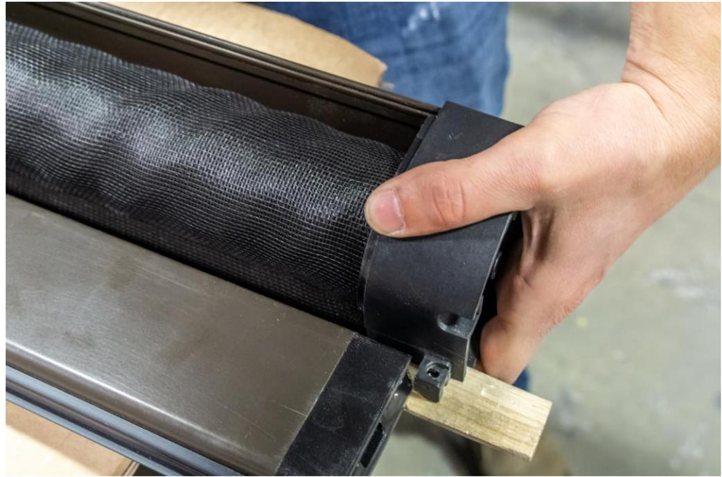
Slide the mesh into the slot into the endcap
