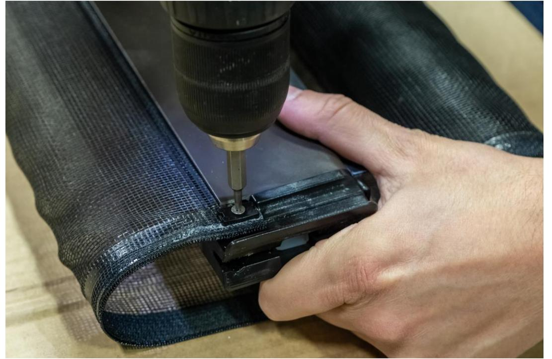
Invert the pull-bar and remove the two mesh retainers
