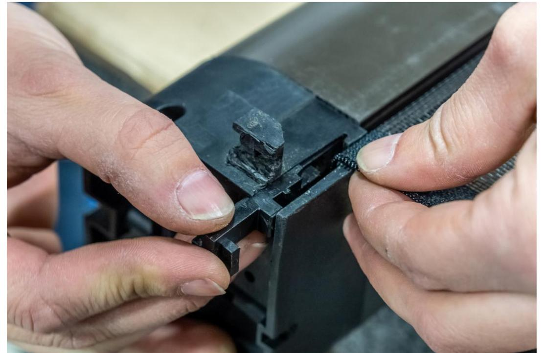
Insert a zip guide making sure the mesh is positioned at the very tip in the wide slot
