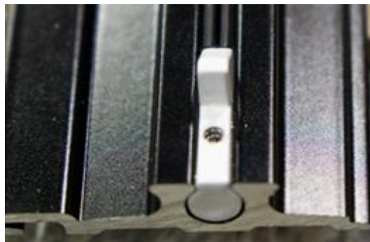
Slide track through pull bar and over housing nipple
