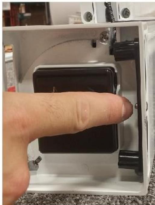
Slide the pull bar onto the mesh spline then tighten the spring
