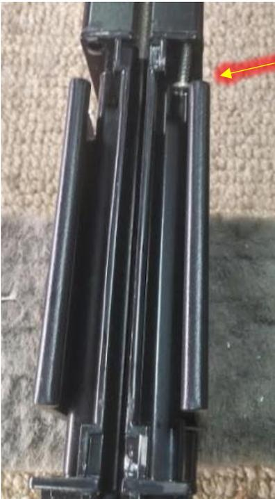
*To rebuild, hook the brake rod onto the Pullbar endcap, insert the endcap into the and re-fasten the 4 screws on one end of the Pullbar*
