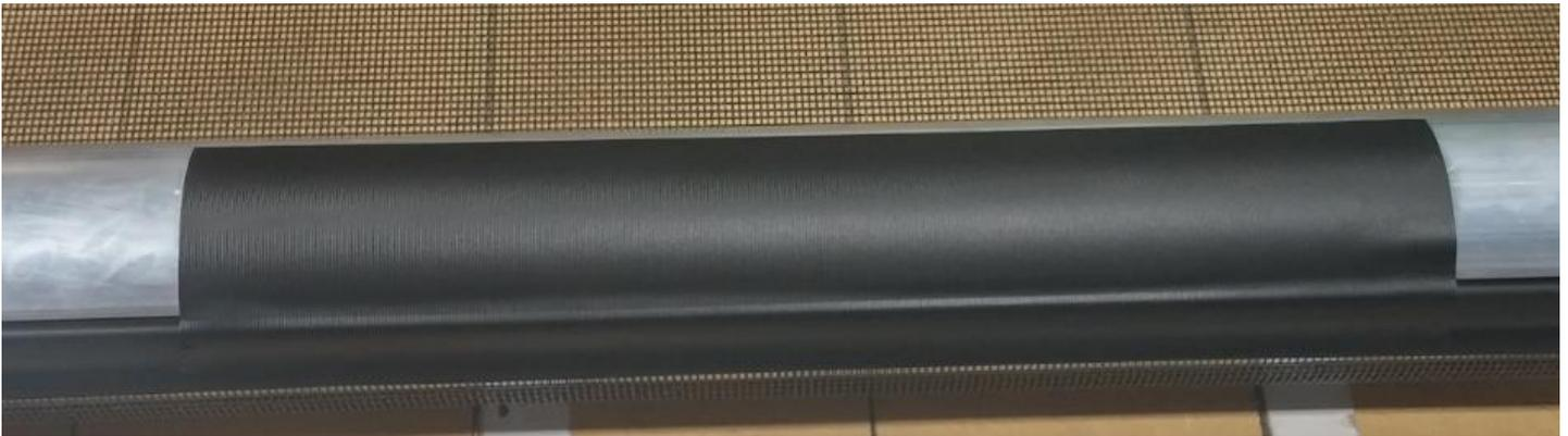
Place the spring in the upper endcap, re-attach the endcaps, and feed the mesh into the endcaps
