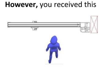
A **RIGHT-HANDED unit** was ordered. <u>But a LEFT-HANDED unit</u> <u>should have been ordered</u>. (See measuring guide).
