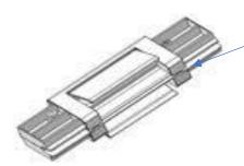
Release the 2mm Allen set screws in the handle – 1 on each side, 1 on the top side, 1 on the bottom side
