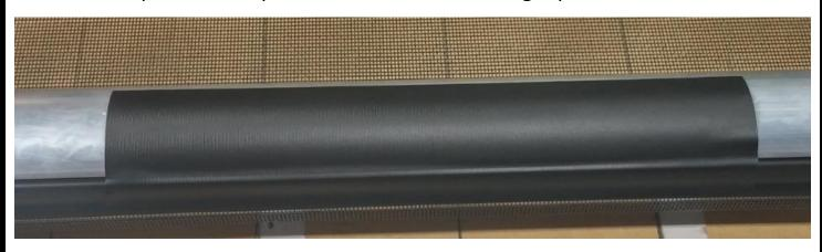
Place the spring in the upper endcap, re-attach the endcaps, and feed the mesh into the endcaps
