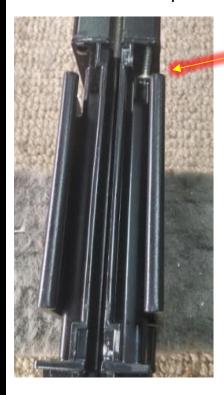
To rebuild, hook the brake rod onto the Pullbar endcap, insert the endcap into the and re-fasten the 4 screws on one end of the Pullbar
