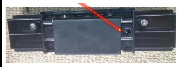
Unscrew and remove the endcaps from the pull bar – 4 screws on each end
