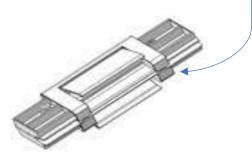
Unscrew the 2 small 2mm Allen screws (one on each side, one at the bottom and one at the top)
