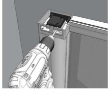
Reinstall the unit. Test by drawing the screen out. Tension may be increased or decreased while the unit is in place if necessary. If possible, request the homeowner operate and adjust to their liking.
