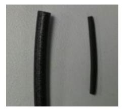
Locate small spline in the channel
