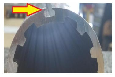
\**Tip* – *Unroll existing mesh and line up new mesh the same way onto roller tube* Overlay the mesh equal amounts on each end of the roller tube
