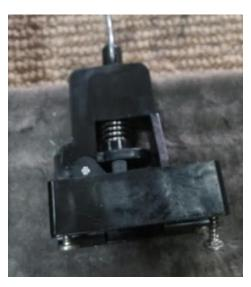
Remove the 8 screws that fasten the handle to the Pullbar, 4 on the top and 4 on the bottom and separate the handle from the Pullbar
