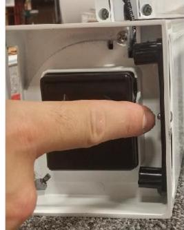
Slide the pull bar onto the mesh spline then tighten the spring
