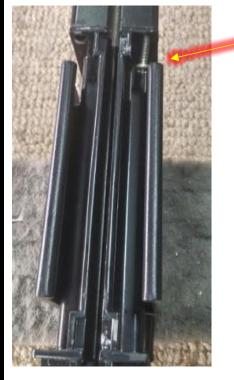
To rebuild, hook the brake rod onto the Pullbar endcap, insert the endcap into the and re-fasten the 4 screws on one end of the Pullbar
