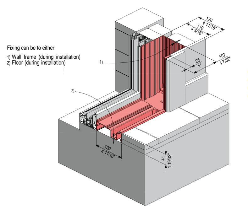
Allow min. 1/4" space between integrated frame and rough frame members for shimming (not shown).
