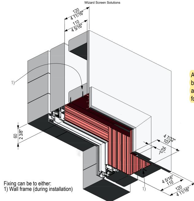
Allow **min. 1/4**" space between integrated frame and rough frame members for shimming (not shown).
