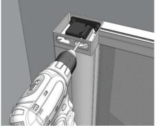
Lay the unit face-up. Increase tension, clockwise at the front.
