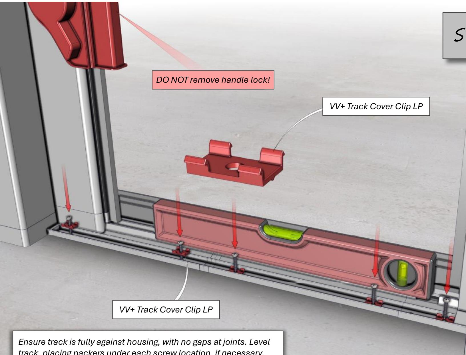
Ensure track is fully against housing, with no gaps at joints. Level track, placing packers under each screw location, if necessary. Secure "Track Cover Clips" with #6 screws into floor.
