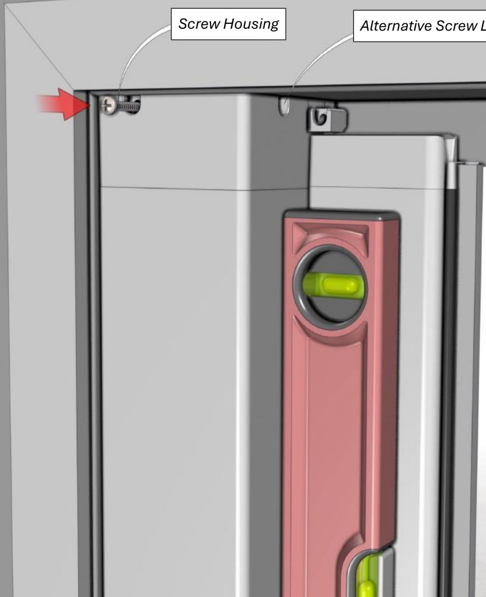
Check "Housing" for level and install one screw to secure as shown.
