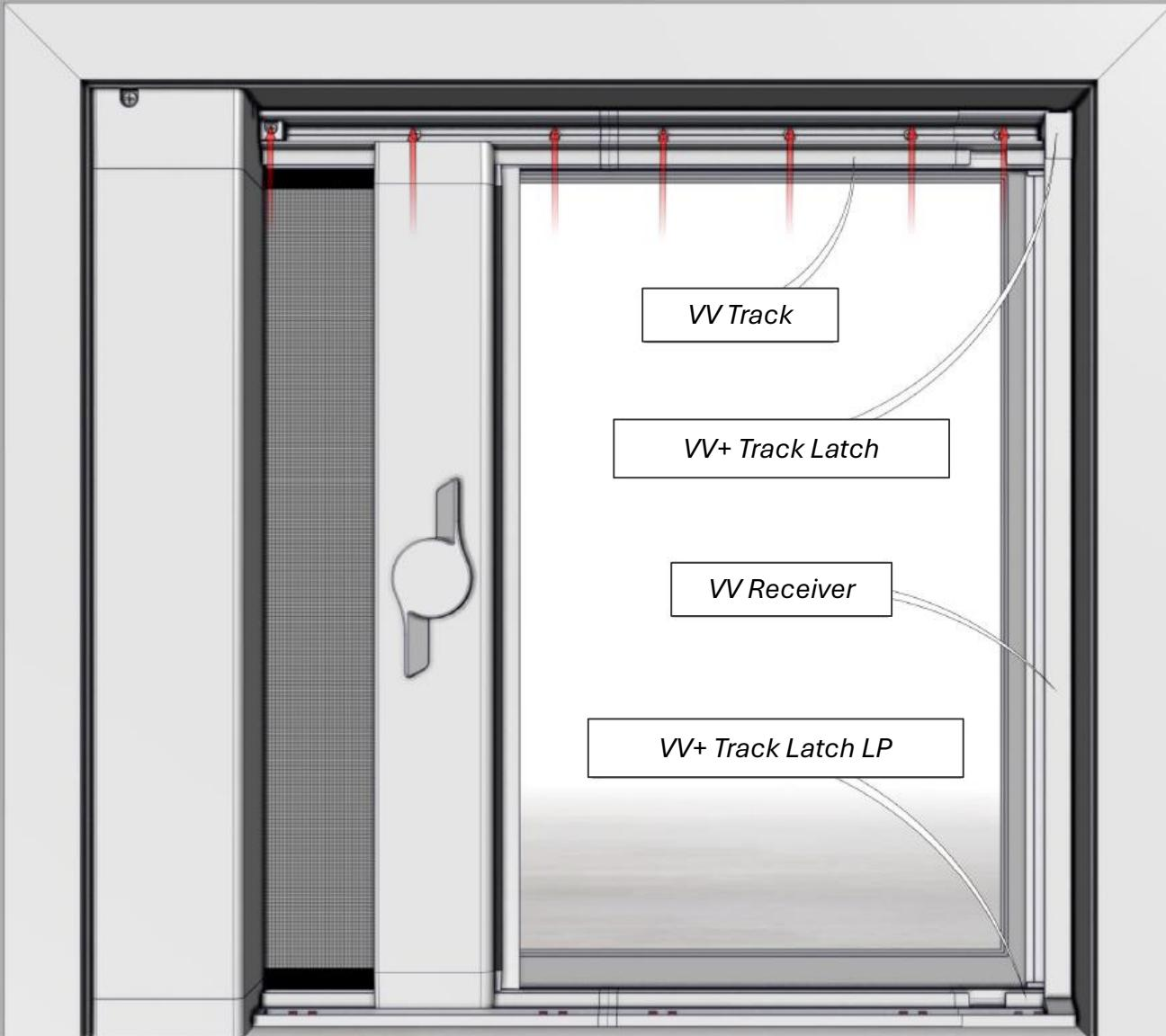
Ensure “Track”, “Latch”, and “Receiver” connections do NOT have gaps, then install remaining screws in upper “Track” and receiver.
