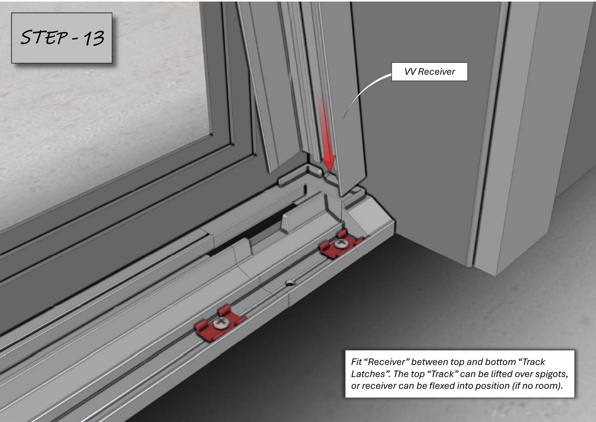
Fit "Receiver" between top and bottom "Track Latches". The top "Track" can be lifted over spigots, or receiver can be flexed into position (if no room).
