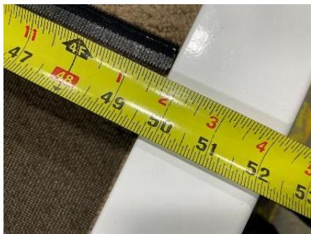
f) Centre **roll-tube** on top of **mesh**. Spacers between **roll-tube** & **straight-edge**.
