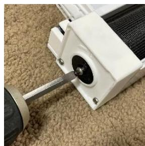
i) Screw both endcaps to housing front using **#6 x 1 ½ panhead screws**.
