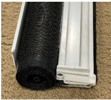
b) Place corresponding **tensioner** "A" or "B" into centre of **bottom end cap** (idler end). Feed onto **zippers** and dry fit to **housing back**, and **speed reducer** into **tensioner**.
