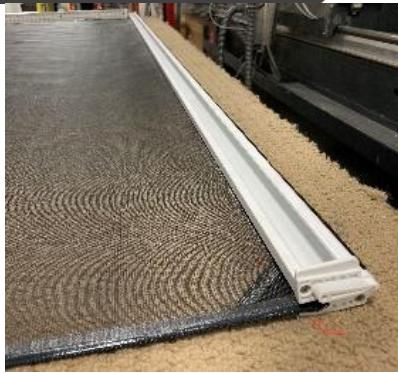
e) Measure out from the **straight-edge** to **pull-bar** at both ends.
