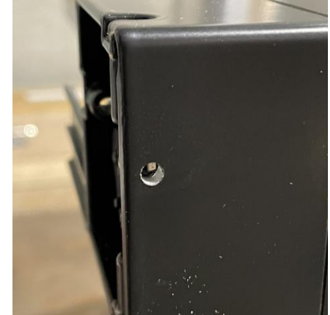
Pre-thread by passing screw in and out.
